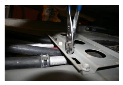
II. Remove the bolts attaching the stock BP using a 12mm socket (4x).
