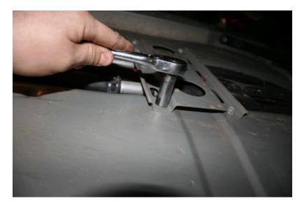
III. Remove the bolts attaching the stock piece using a 12mm socket (2x).
