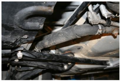
III. Put the FMB in place as shown and hand tighten the mounting bolts to hold it in place (4x).
