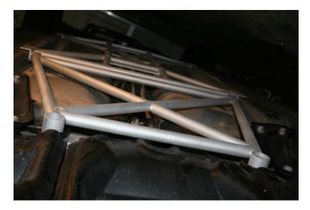
IV. Snug the mounting bolts using a 17mm socket (4x).
