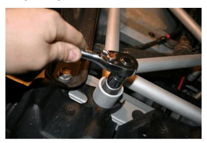
V. Torque the mounting bolts to 55 ft/lbs (4x).
