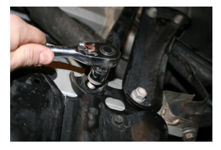
II. Remove the stock rear a-frame bolts using a 17mm socket (2x). Note: if you are not using the MSMB as shown you will need to install the spacers provided. Otherwise they are not necessary.
