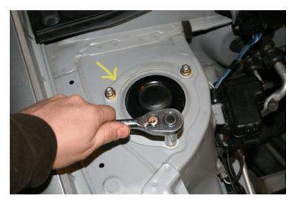
III. Place the FSTB in place with the Cross Bar and welds facing up. It may fit rather snug so push one side down a few threads, then the other equally. Repeat this until you walk each side to the bottom of the threads. This may require lateral movement of the car and/or brace to achieve (slightly rock the car by the fender). Take special care not to hammer the brace down, thus potentially damaging the threads of the bolts.
