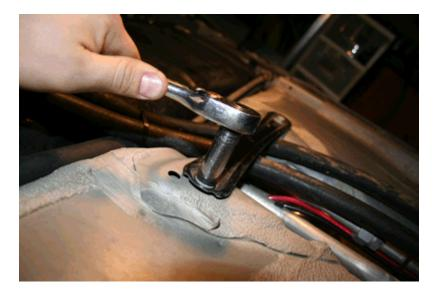
IV. Remove the small bolts about 12" to the outside of the car using a 10mm socket (2x). Directly across from the rear stock BP bolt location.
