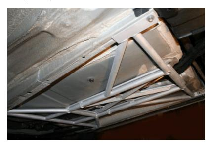
VII. While holding the MSMB in place, loosely tighten two bolts, one each in 2 opposite corners of the BP location using the supplied bolts and washers (to hold the MSMB in place).
