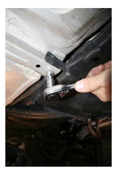
V. Remove the rear bolts of the front A-frame brace using a 17mm socket (2x).
