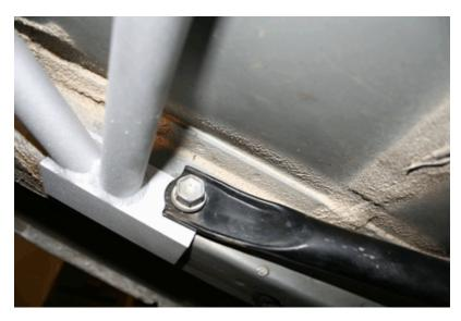
X. Insert the rear 10mm bolts and hand tighten (2x).
