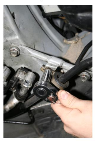
II. Remove the bolts from each dog bone brace using a 14mm socket (2x).
