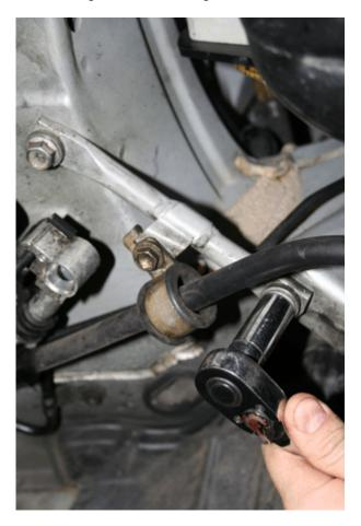
III. Put the RLCB in the position as shown below and hand tighten the 4 bolts to hold it in place. However, unlike the picture, the brake line goes on top of the brace as it did on the stock dog bone brace (thus the threaded hole).
