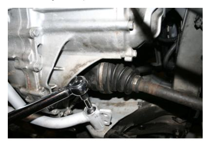
X. Remove the upper strut rod bolt for the RMB extension braces installation.
