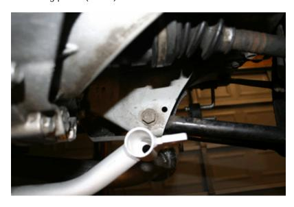
V. Remove the bolts from the rear mounting location using a 17mm socket.
