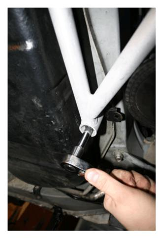
IV. Snug the gas tank bolts just enough to raise the rear of the brace as shown in the picture below. The RMB should now be hanging from the rear gas tank bolts with just enough slack to expose the rear mounting points (12mm).
