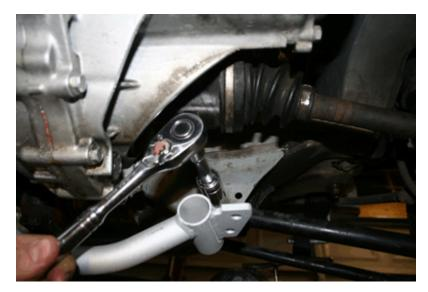
VI. Reinsert and hand tighten, repeat on the other side. You may find it necessary to push out on the wheel to get the bolt back in place. In fact, it is a good idea to put some pressure on the wheel while removing the bolt to prevent it from slipping out of position when the bolt is removed.
