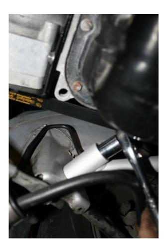
XIII. Use the supplied nut, bolt, and washers to connect the RMB extension to the RMB x2.
