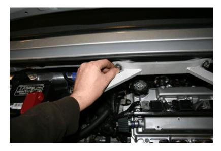
VIII. Tighten all, firmly with a ratchet and 14mm socket (6x).
