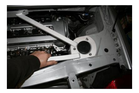
VI. Hand thread the nuts back on the bolts of each strut tower, remember the washers on the 2 inside nuts (6x).
