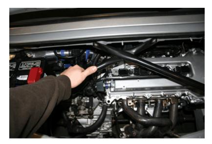
V. Place the RSTB in place with the Cross Bars and welds facing up. It may fit rather snug so push one side down a few threads, then the other equally. Repeat this until you walk each side to the bottom of the threads. This may require lateral movement of the car and/or brace to achieve (slightly rock the car by the fender). Take special care not to hammer the brace down, thus potentially damaging the threads of the bolts.
