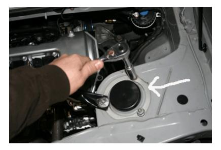
III. Remove the upper bolts from the stock X-Brace (2x).
