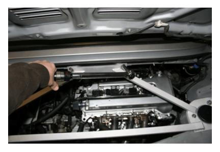
X. Torque the strut tower bolts to 59 ft/lbs (6x)
